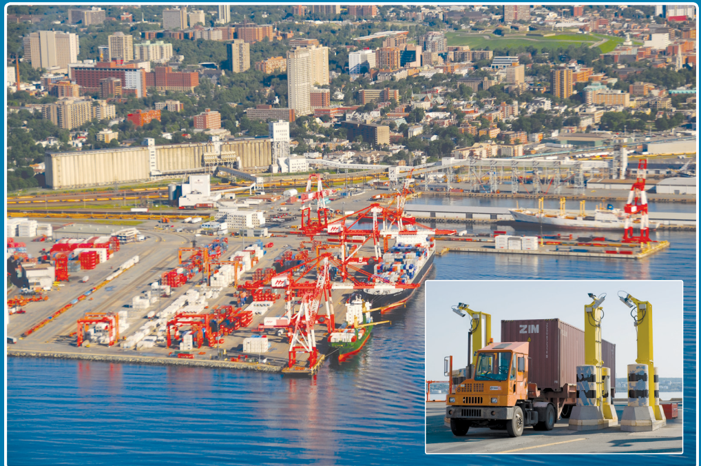
At the Halifax Port Authority's South End Container Terminal, a container is scanned by a radiation detection portal.
