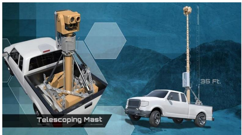
The system mounts to the bed of any 5 x 6’ pickup truck, offers an unprecedented 35-foot-high vantage point with high resolution thermal and day cameras for detection and identification.
