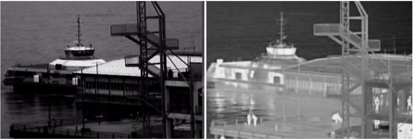
Figure 5 – Detection: Visible versus Thermal Cameras
