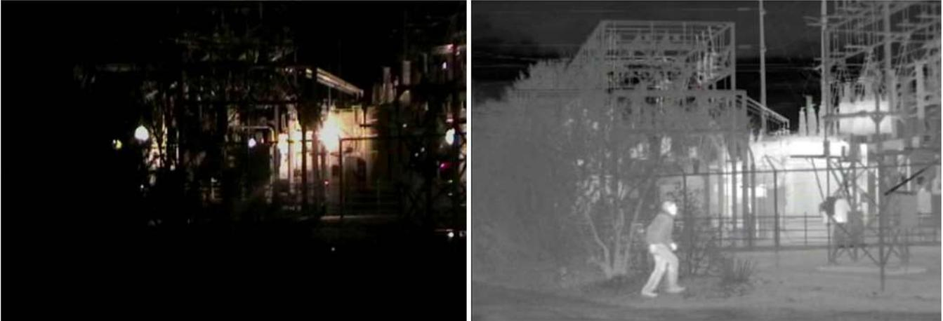
Figure 4 – Detection: Visible versus Thermal Cameras
