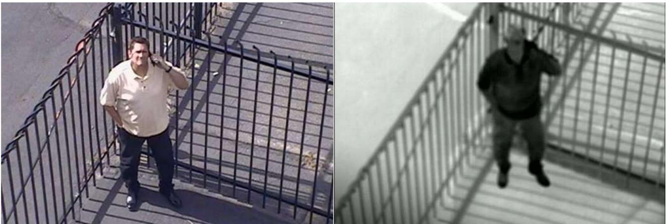
Figure 1 – Identifying: Visible versus Thermal Cameras
